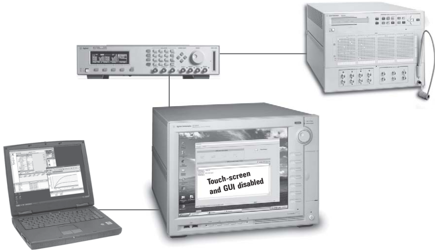
Figure 9. B1500A using an external PC to control analyzer measurement resources and external GPIB instruments. The built-in PC controller, touch-screen and GUI are disabled.
